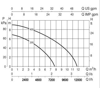
$\label{eq:main} The performance curves are based on kinematic viscosity values = 1 \ mm^2/s \ and \ density \ equal \ to \ 1000 \ kg/m^3. \ Curve \ tolerance \ according \ to \ ISO \ 9906.$
